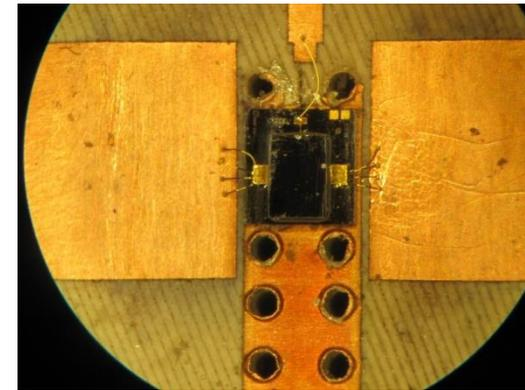
*Microscopic image of an RF MEMS switches used on a reconfigurable resonator*
