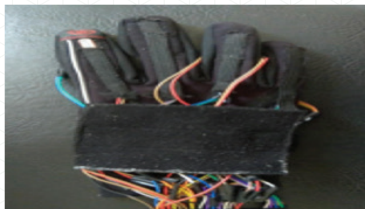
Figure 2: An instrumented passive glove
