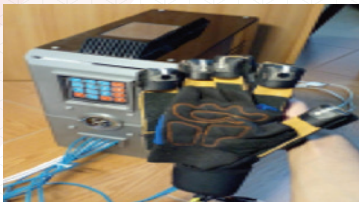
Figure 1: A soft robotic actuated glove
